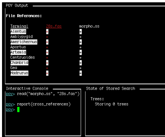
Figure 2.23: Visualizing missing data. The command cross_references displays a table showing whether a given terminal (in the left column) is present (“+”) or absent (“-”) in each datafile. In this example, the data for all the taxa listed in the POY Output window are present in both datafiles, morpho.ss and 28s.fas .
