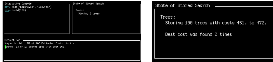
Figure 2.24: Generating Wagner trees. During the process of tree building (left panel), the Current Job window displays how many builds have been performed so far (57 of 100), the number of terminals added in the current build (13 of 17), a cost of a current tree recalculated after each terminal addition (362), and the estimated time (in seconds) for the completion of the operation (4 s). Because the process is not complete, the State of Stored Search window contains no trees. Once tree building is complete, the State of Stored Search window displays the best (451) and worst (472) costs, the number of trees stored in memory (100), and the number of trees with the best cost (2).
